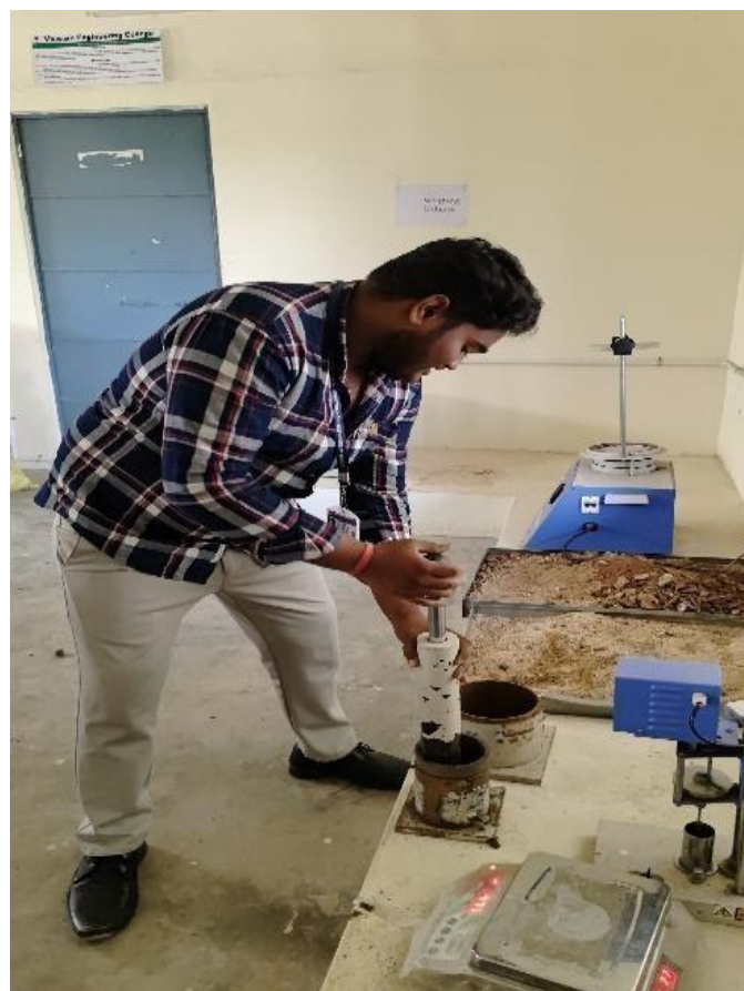
Fig.3 Standard Proctor Compaction
