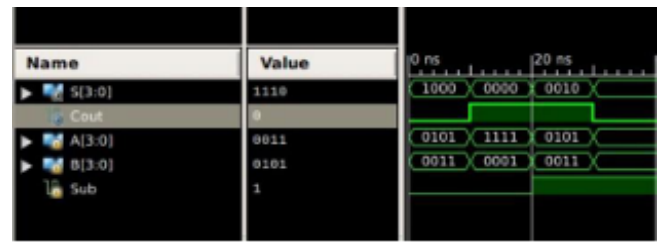
Fig.5 The result waveform of the CLA adder and subtractor in Binary format
