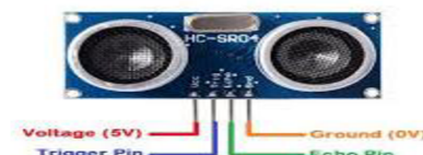
Figure.1: Ultrasonic sensor module consists of 4 pins
